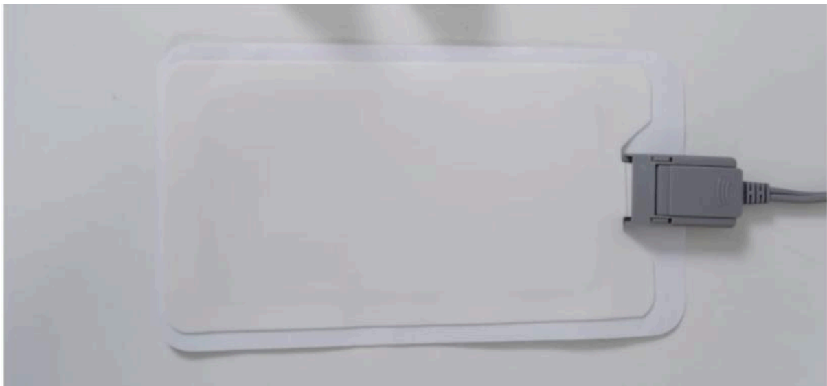
Figure 19. Rejera® return electrode, responsible for closing the monopolar radiofrequency circuit and ensuring safe current dissipation.
